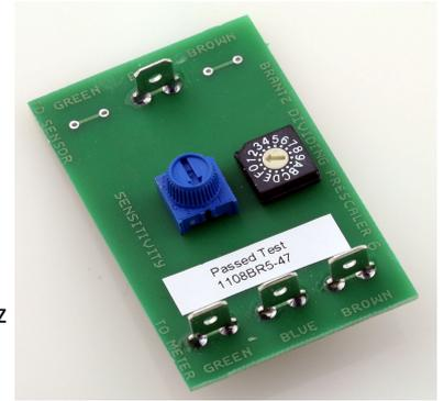
The rotary switch on the interface sets the pre-scale ratio/dividing multiple i.e. set on 2 it will divide the number of pulses from the vehicle to the Brantz Meter by 2. **It should initially be set on 1.**
